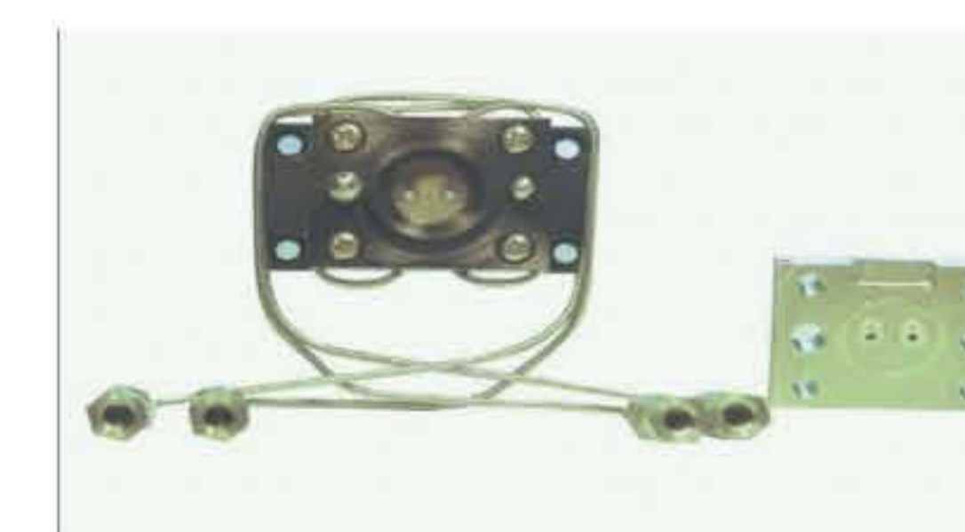
The heart of UV detector: flow cell
